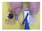
Remove the four tiny screws holding the printed circuit board and battery retainer to the white plastic inner case. Remove the electrically conducting pad and the LCD panel. Place the screws, switch contacts, and battery contacts into a small container for safe keeping.
