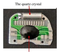
The integrated circuit chip is sealed in here.
