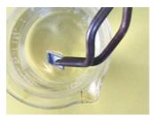
When a liquid crystal melts, the molecules become less ordered and the display appears black. The change is reversible if the heating is not too severe.
