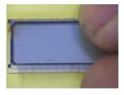
Examine the LCD panel and find the contact area of the panel on the bottom of the wider glass plate. Use a battery cap connected to 9-V battery. Hold one of the leads against the contact area at one end of the panel and rub the other lead along the contact area to address various segments of the LCD panel. Record your observations.
