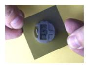
Hold a piece of polarizing film over the watch display. Slowly rotate the polarizer above the LCD panel. Does the orientation make a difference?
