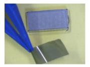
This step is not totally reversible. Remove the top polarizer by carefully prying up one corner and then gently peeling it away.
